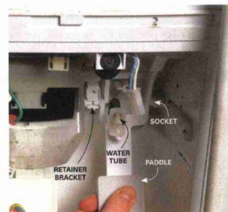
4 INSTALL A NEW PADDLE Remove the metal retainer plate (not shown). Replace the broken paddle with a new one. Reattach the water tube.
