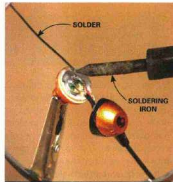
2 SOLDER THE CONNECTION Place the wire on the circuit board and hold it in place with the tip of the soldering iron. Add solder. Then remove the hot iron and hold the wire in place until the solder cools.
