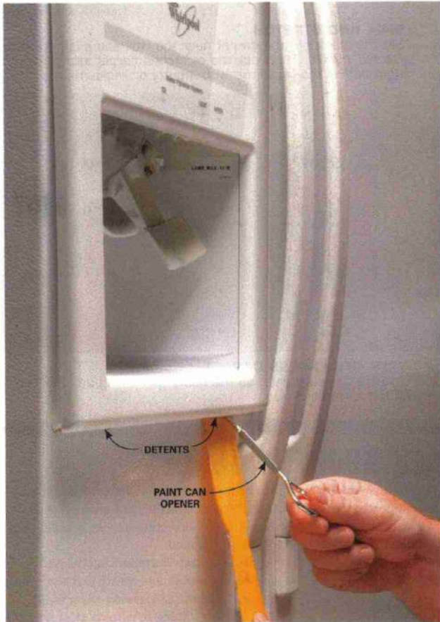
1 REMOVE THE TRIM PANEL Locate the detents in the trim panel. Slip a plastic putty knife up against the trim and wedge off the trim with a screwdriver or paint can opener.
